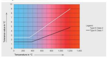
Example: Tolerance value of the accuracy classes 1 and 2 of thermocouple type K
